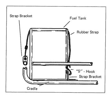
Check that both the 5 gallon fuel tank and its rubber strap have been received. The rubber strap has an "S" -Hook at each end that inserts into strap brackets on the alternator cradle.
